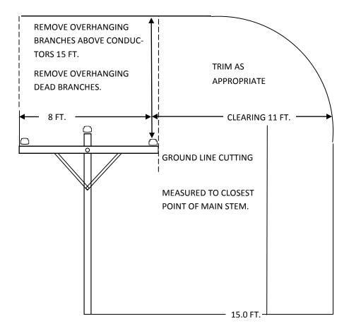
ALL DISTANCE ARE MEASURED FROM OUTERMOST PRIMARY CONDUCTOR.
