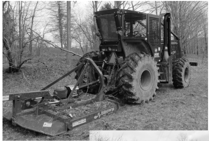
New mowing machine and example of cleared Right-of-Way.
