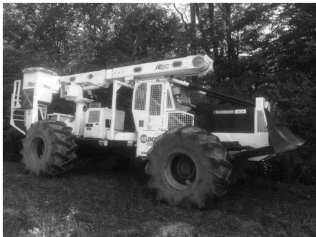
Used in off-road portions of the ROW. A crew member uses the bucket in an elevated position to trim branches of trees growing in from the side of the ROW toward the electric lines.
